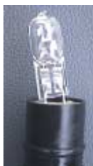
Incorrectly seated halogen bulb
